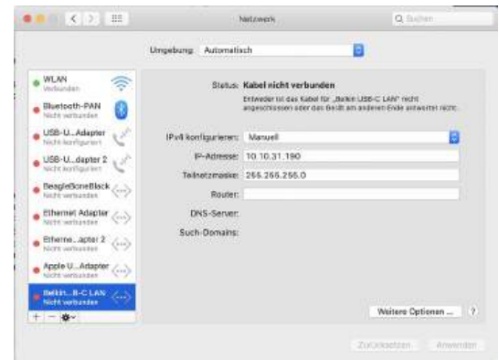
Figure 6: IP configuration of a USB-LAN adapter
