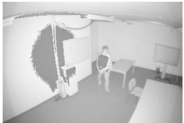
Figure 4: Amplitude as logarithmic gray scale
